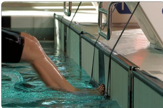
The backstroke ledge improves the start push and trajectory of the swimmers when they enter the water
